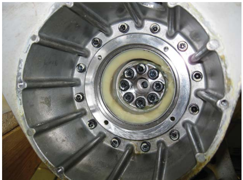
Same Axis & Robot As Above, Cleaned, Greased and Reassembled
